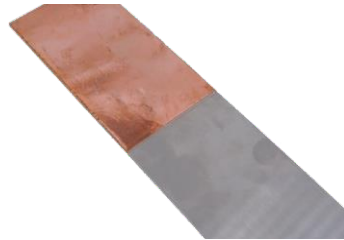
Welding of blue light composite red copper with stainless steel
