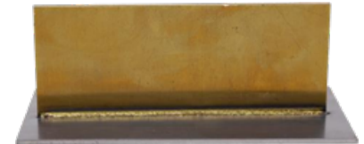
Welding of brass with stainless steel
